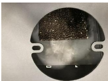
Catalyst assembly seen from the flue outlet above the vermiculite flue baffle
