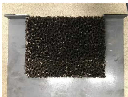
Catalyst assembly seen from the flue outlet above the vermiculite flue baffle
